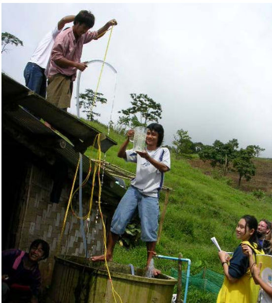
Measuring flow with 3 m head.
